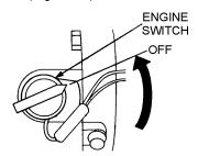
Figure 15. Engine ON/OFF Switch (OFF)
